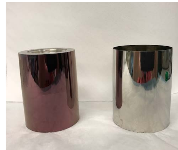
Mandrel ( left ) and replicated NiCo optic ( right )
