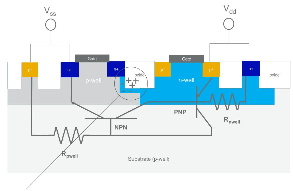
Positive charge build-up in oxide creates low resistance pathways that allow n+ to n-well leakage
