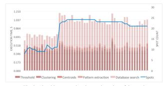
Fig. 2. Algorithm execution time and number of detected spots
