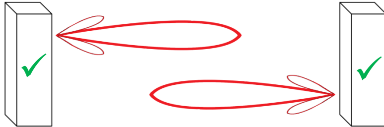
Directive antennas for normal operation
