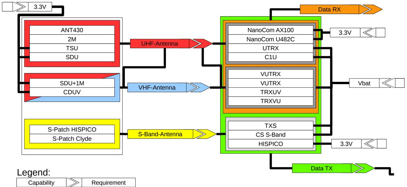
Figure 3: Diagram of Example Components, their Requirements and Capabilities.
