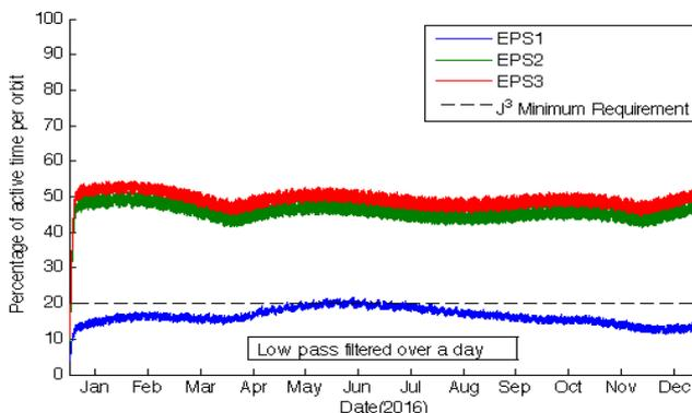
Figure 5: Impact of EPS efficiency on available instrument measurement time
