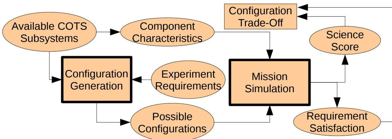
Figure 2: Workflow Diagram of the Design Process for J<sup>3</sup>
