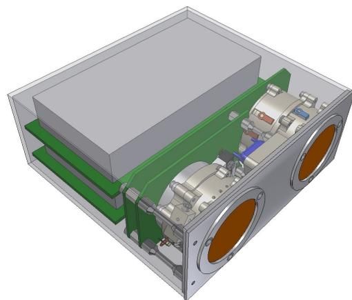
Figure 1: Model of the Radiation Test Experiment for JUICE (RATEX-J)
