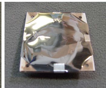
Ant Dev Corp Medium Gain X-band Patch Array Antennas • 2.5X2.75X0.13 inches
